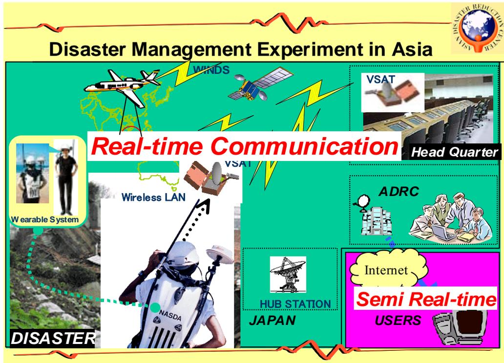
Fig.2-8-4 Disaster information system that utilizes Wideband InterNetworking engineering test and Demonstration Satellite (WINDS)
