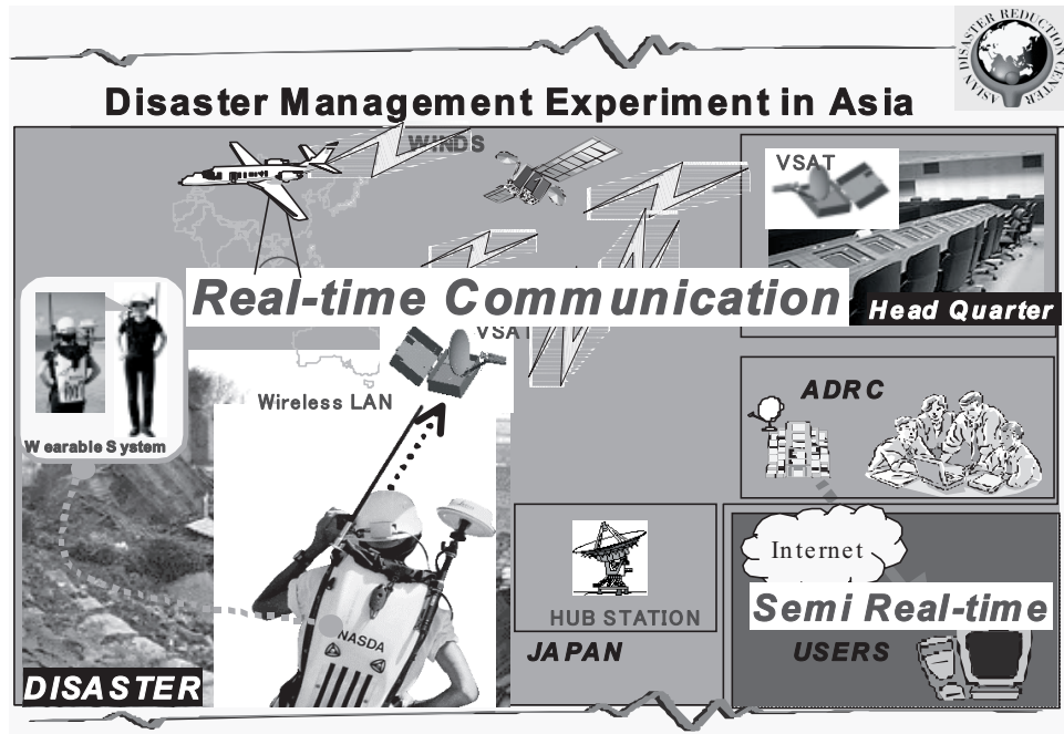
Fig. 2-8-3 Realtime Disaster Information System by communications satellites
