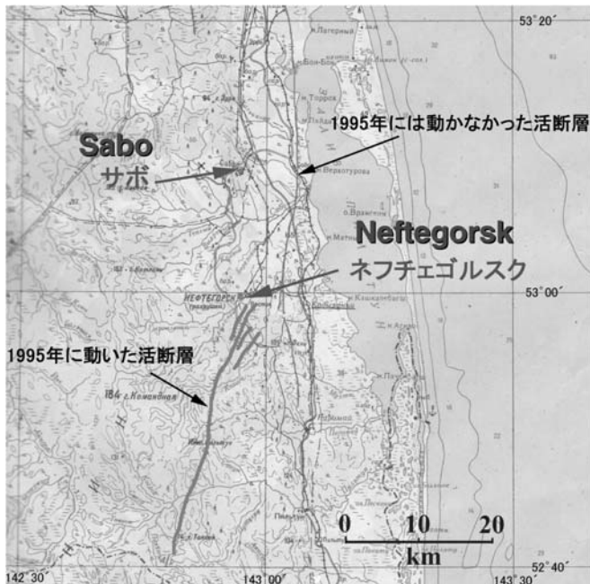
Figure 1. Distribution of active fault from which an earthquake occurred in Sakhalin 1995: The town of Neftegorsk was totally destroyed though Sabo was sound
