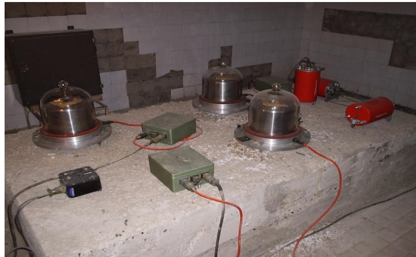
Fig.5. Seismic sensors installed in Garni
