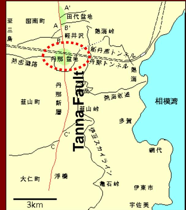
This earthquake led engineers to consider effect of faults crossing tunnels
