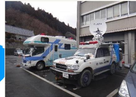
Securing a communication circuit with a satellite communication vehicle
