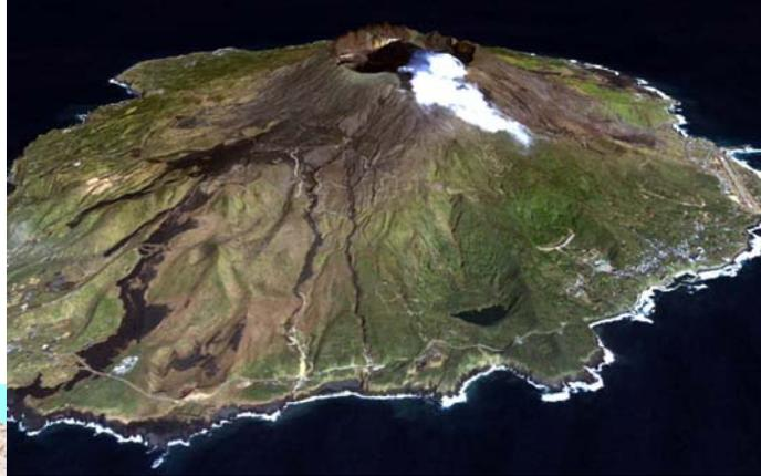
3D view of Miyakejima Island generated by overlaying PRISM DSM with pan-sharpened image of PRISM and AVNIR-2. Mar. 1, 2007.
