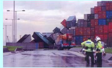
Stacked containers collapsed in a Container Terminal due to a gust front on 9 May 2005
