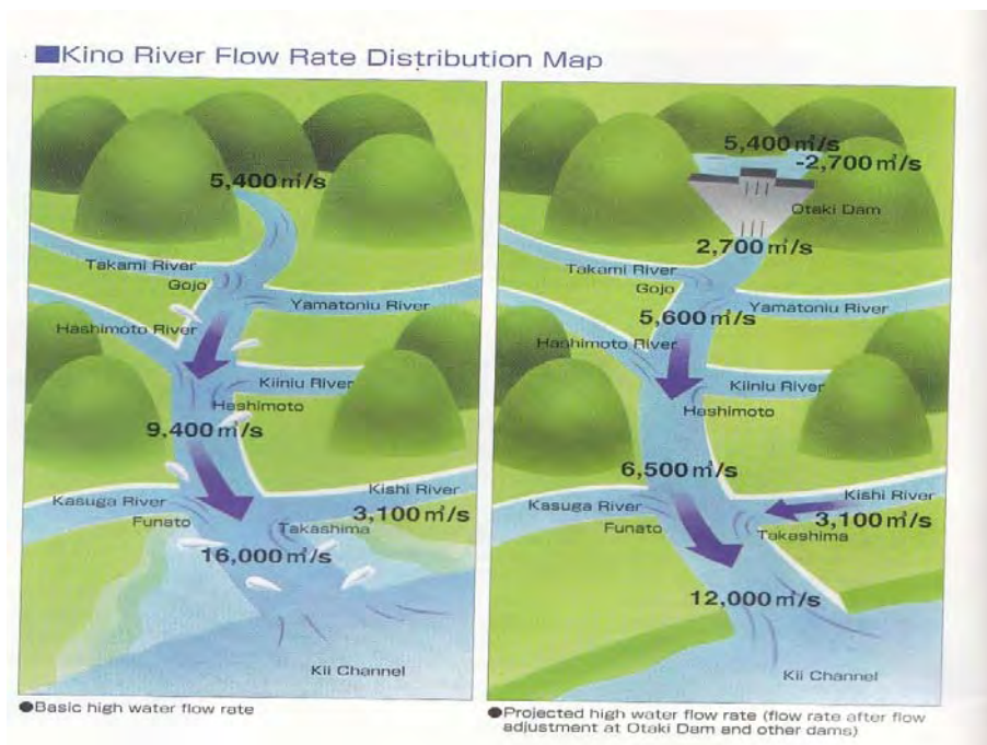
Figure shows Flood control system of Kino River, Japan using a flood control Dam
