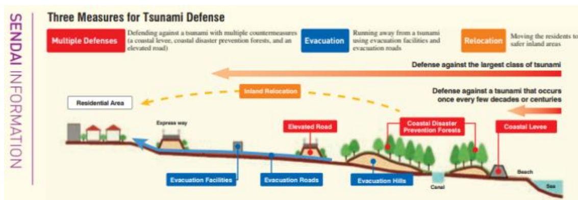
Figure 27: Three measures for tsunami defense (Source: City of Sendai)
