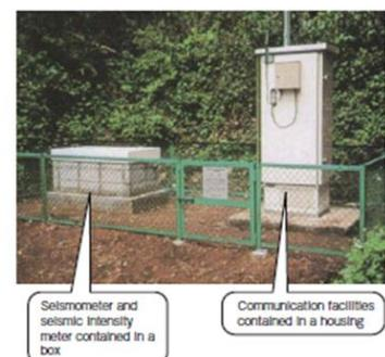
**Figure 23: JMA Seismic station**
