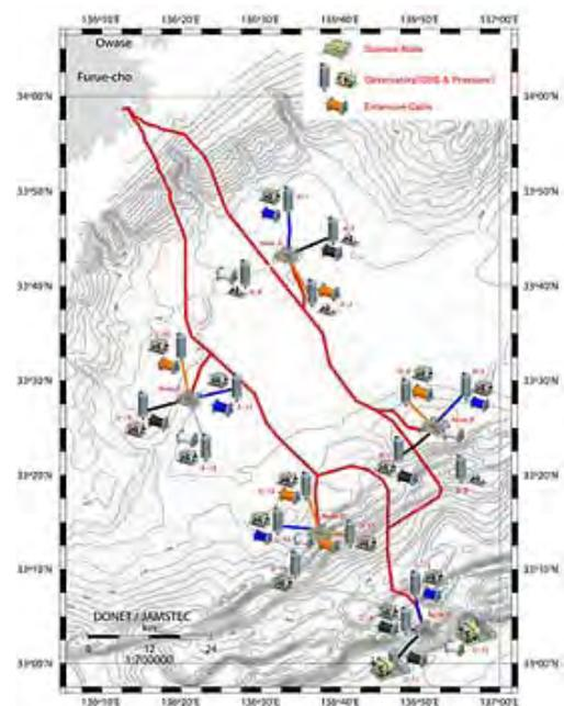
observatory network for the precise earthquake and tsunami monitoring. For the purpose of understanding and forecasting the earthquake and related activities underneath the seafloor, the twenty sets of state-of-arts submarine cabled sub-sea measurement instrument will be deployed in seafloor at the interval of 15-20km. The twenty sets of preliminary interface are prepared in consideration of the improvement of observation capability in the future. Operating
