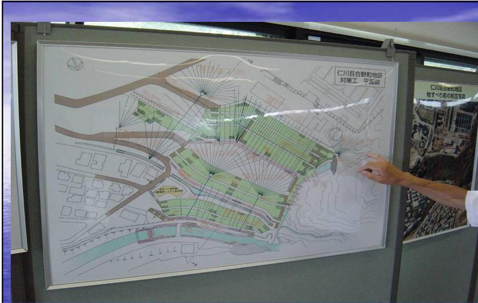
Many pipes constructed to drain the land in conducting Landslide prevention
