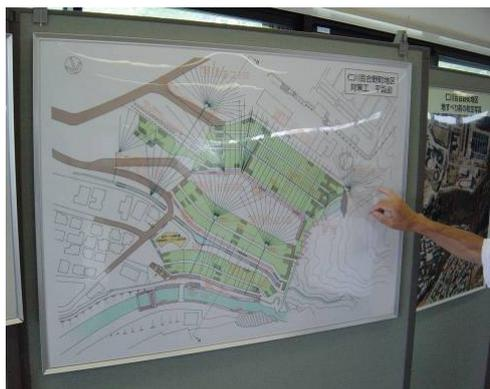
Many pipes constructed to drain the land
