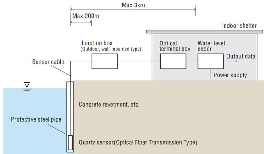
**Figure 2.14. Configuration diagram**
