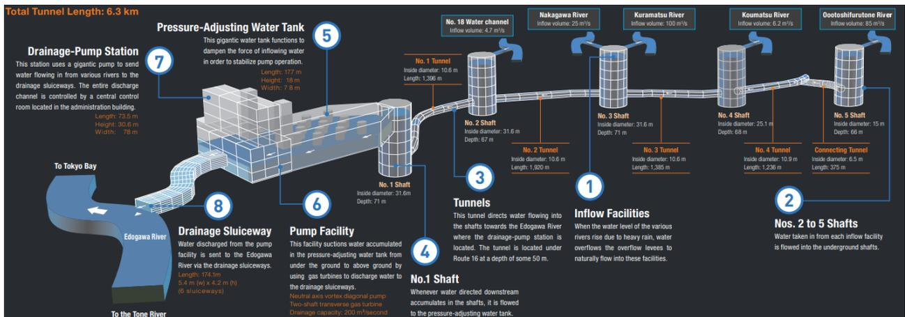
Figure 2.35. Mechanisms of the Metropolitan Outer Area Underground Discharge Channel
