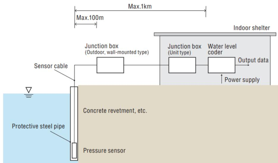
**Figure 2.17. Configuration diagram**
