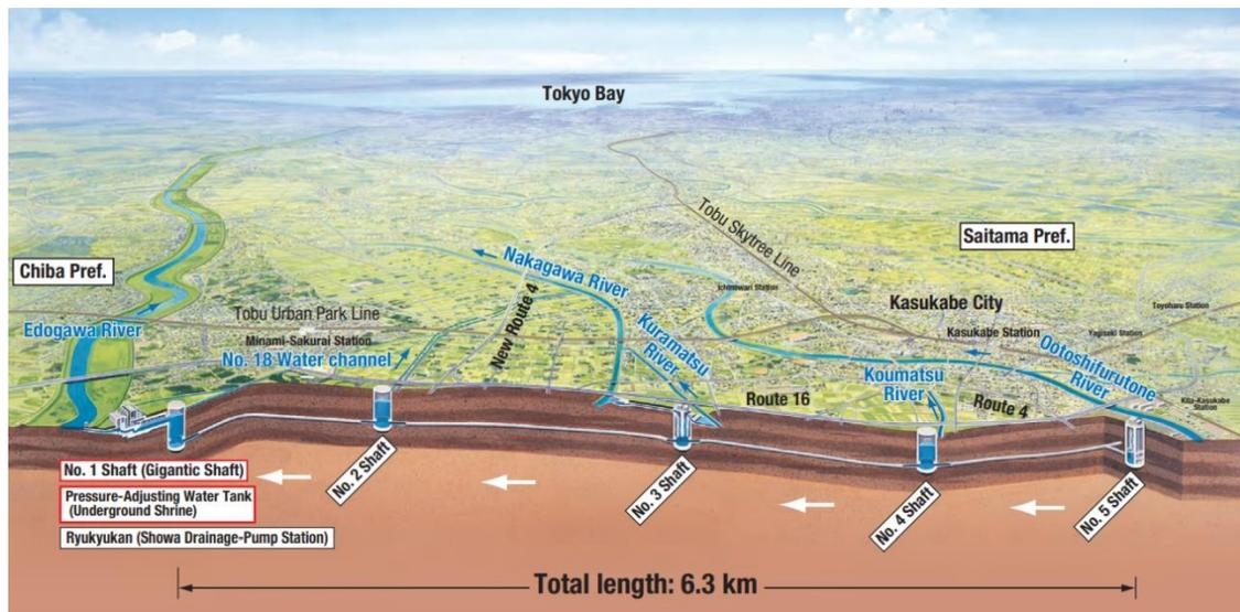
Figure 2.32. Structure of the Metropolitan Outer Area Underground Discharge Channel
