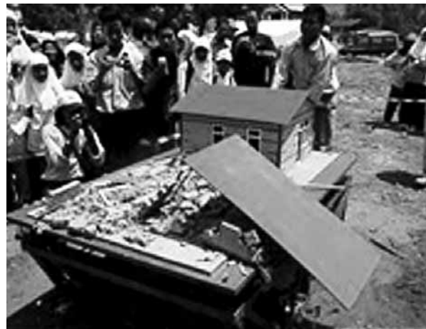
Fig.4-2-2-2 "Shaking Table" demonstration using typical model for local housing
