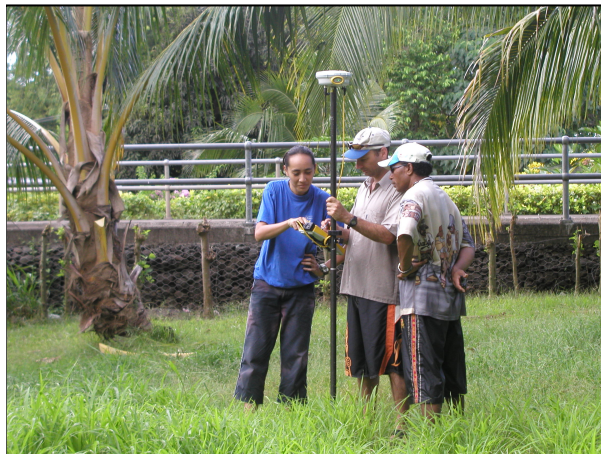
River transect across the floodplain using RTK GPS
