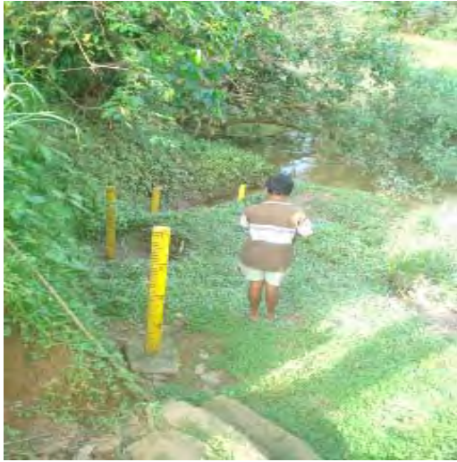
Figure 8.11: Water Level gauge at Thunthota, Kegalle District maintained by Irrigation Dept.
