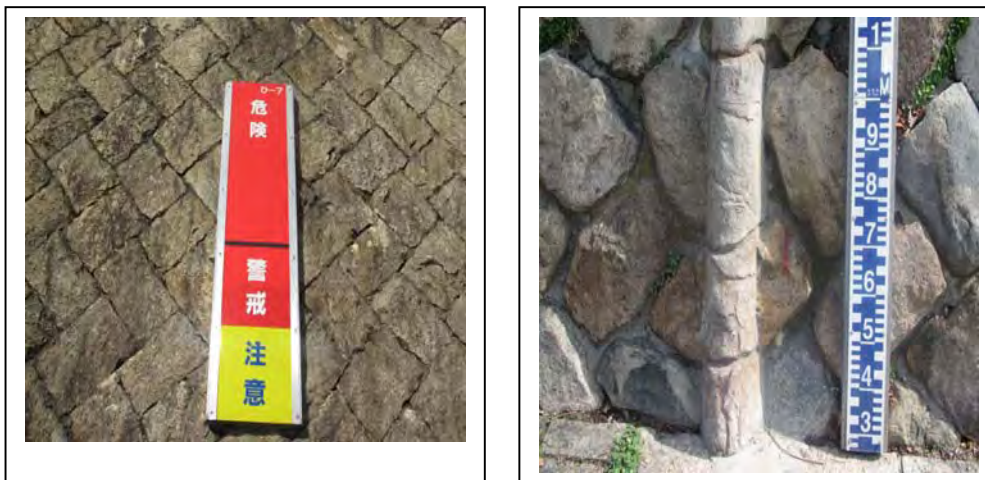
Figure 7.14: Water level measuring gauges and senses fixed to the river banks
