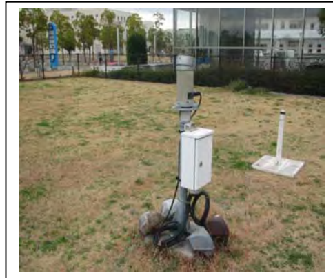
Method for Observe Weather Condition (Small rain drops, snow...) – Can not measure the amount
