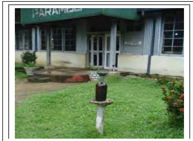
Figure 8.9: Rain Gauge operated by rubber Plantation (one at Parambe estate, Kegalle District)
