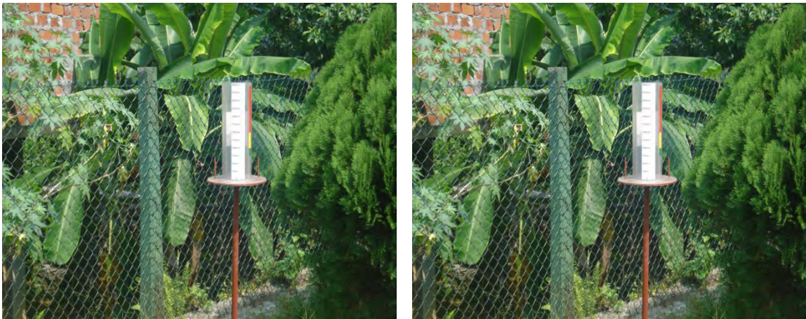
Figure 8.10: Normal Rain-gauges distributed by Disaster Management Centre (one at Bulathkohupitiya Divisional Secretariat, Kegalle District)
