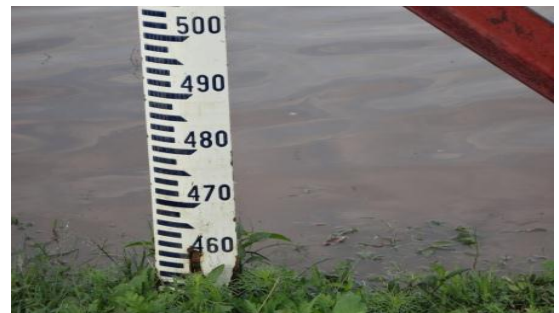
Manual River Gauging Station & monitor
